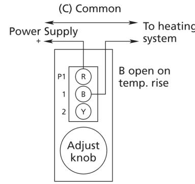
Figure 1 – Connection for a Typical Heating Control Circuit
